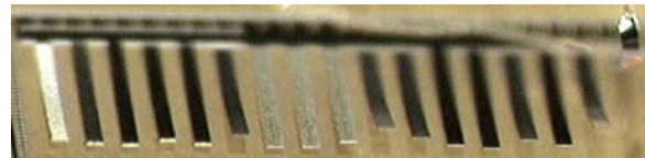
Fig. 3. Photomicrograph of fully released cantilever beams
