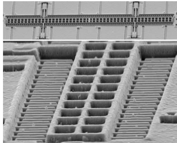
Fig. 5. SEM photographs of entire (top) and close-up (bottom) of magnetometer
